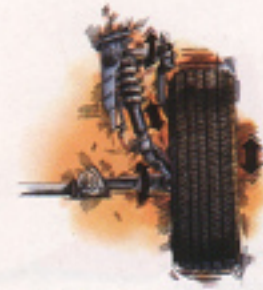
A fully independent double-wishbone touring suspension is among the most sophisticated designs in the world.
